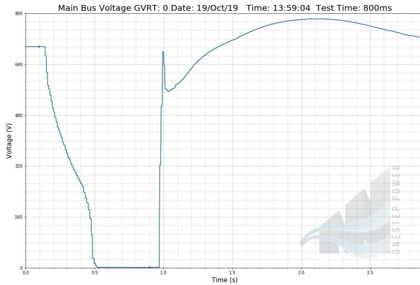
Figure 34. Results of Test 12, Bus A: Pass (800ms)
