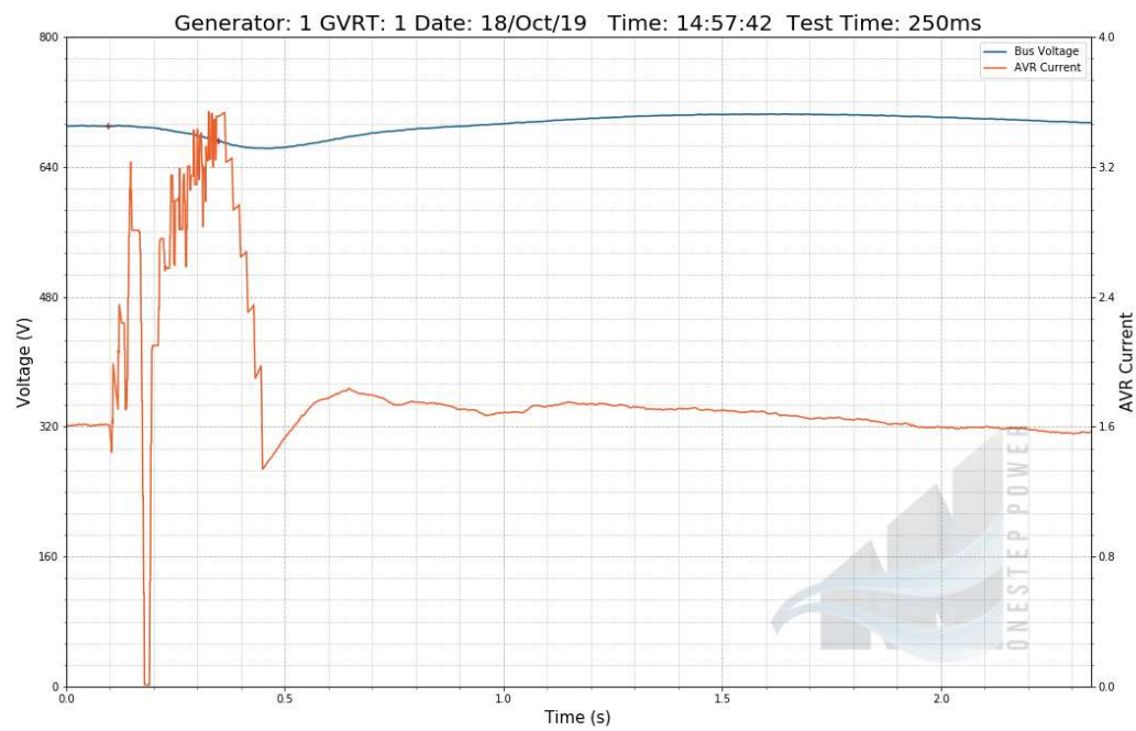
Figure 20. Results of Test 01, Generator #1 250 ms open bus
