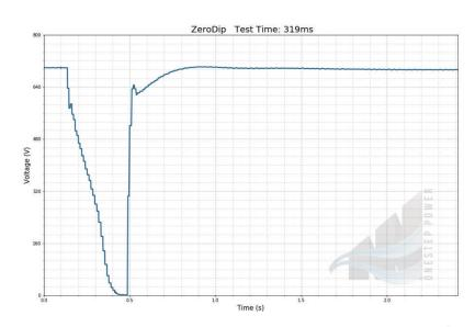
The graph to the left displays the main bus voltage collapsing to zero then returning to rated voltage in a live test conducted on a vessel in service. ZeroDip testing can be completed dockside, prior to sea trials, allowing for early identification and efficient rectification of power distribution system deficiencies.
